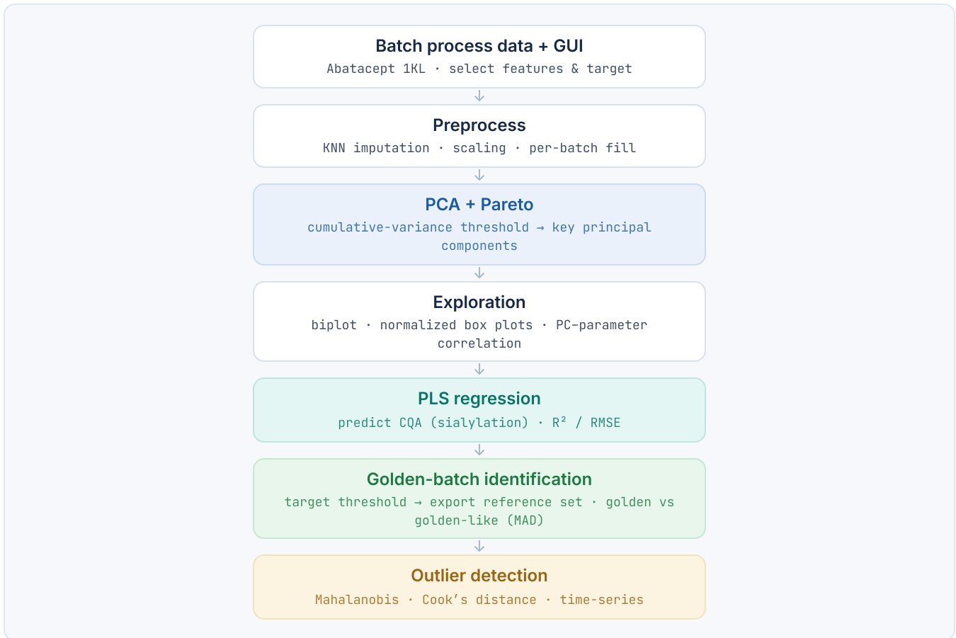
FIG. 01 Analysis pipeline — impute, reduce with PCA, model the quality attribute with PLS, then isolate golden batches and outliers
